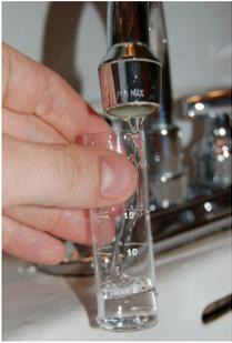
1. Fill measuring tube with 5ml of water from water line going to machine, before installing filter.
