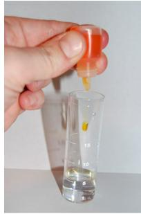
2. Add indicator solution drop by drop. COUNT the drops. Gently mix between drops.
